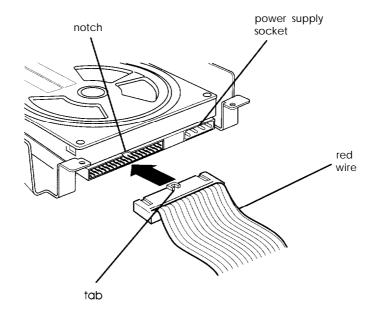
When the hard disk drive ribbon cable is positioned correctly, the red wire on the cable is aligned with pin 1 on the drive connector. To identify pin 1, look for a 1 or 2 at the connector on the drive's circuit board.
